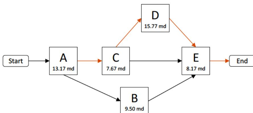
Figure 13.2: AON Network Diagram
