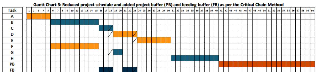
Figure 18.1: Critical Chain Method Gantt Chart
