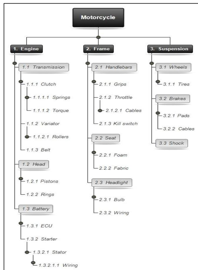
**Figure 11.1:** Product Breakdown Structure
